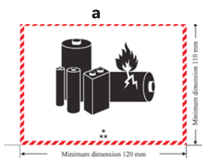
Figure 1 - Labels used in shipment of lithium batteries
