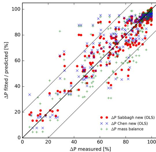
Fig. 2: Measured  $\Delta P$  vs.  $\Delta P$  fitted with the Sabbagh and Chen eqs. (OLS) and  $\Delta P$  predicted with the mass balance approach for the full test data set ( $n = 244$ )
