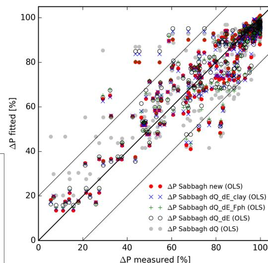
Fig. 3: Measured  $\Delta P$  vs.  $\Delta P$  fitted with the full and the four reduced Sabbagh equations (OLS) ( $n = 244$ )
