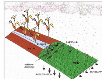
Fig. 1: Schematic representation of a VFS. <http://abe.ufl.edu/carpenna/vfssmod/>
